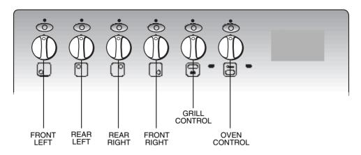
**Control Knobs** The knobs for the grill and hotplates can be rotated in either direction to provide variable heat control, the oven knobs can only be rotated clockwise from the **Off** position.
